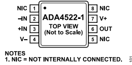
Figure 3. ADA4522-1 Pin Configuration
