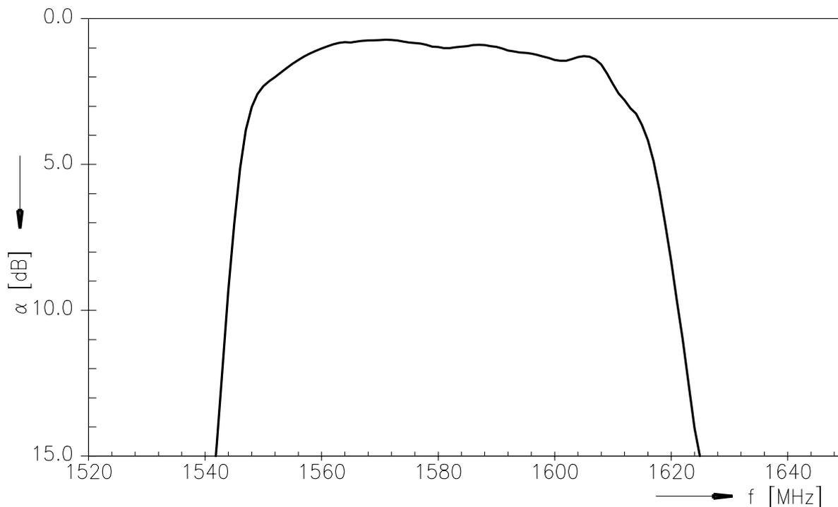
**ANT-BeiDou/GPS/Glonass (transfer function wideband)**
