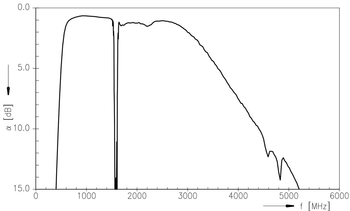
**GPS-CELL (isolation, transfer function)**
