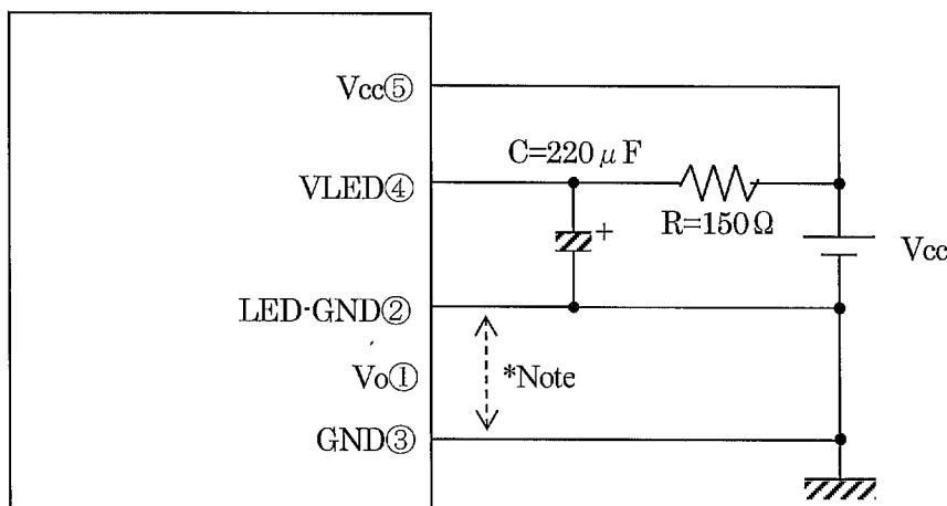
\*Note : LED-GND line and GND line must be separated.
